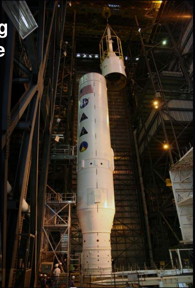
Stacking of the Ares I-X rocket at the Kennedy Space Center Vehicle Assembly Building as depicted by the final element being placed atop the Ares I-X Flight Test Vehicle (FTV) integrated stack.
