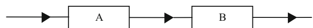
Fig. 1 “Series” combination of two components A and B , where the ability of B to do anything useful relies on the correct functioning of A . The combination only functions correctly if both A and B are functioning normally. The arrows indicate the sequence of any dependency, e.g. of data flow
