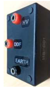
Figure 1. Capacitive Bushing Model
