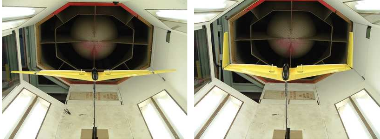
Figure 3. Experimental model as mounted in the wind-tunnel; left: both winglets planar; right: both winglets upright.
