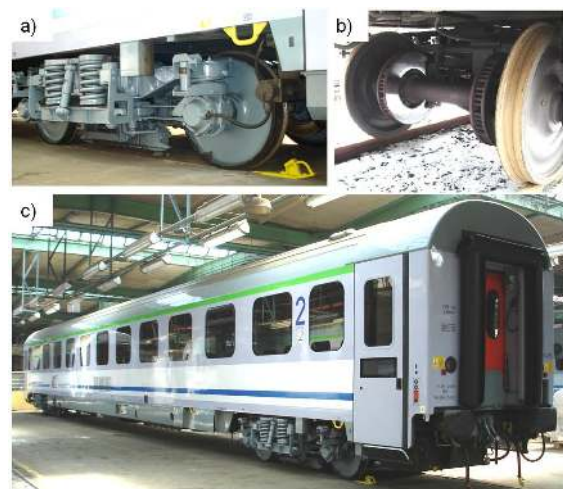
Fig.1. View of the passenger coach fitted with a disc brake: a) view of the MD 523 bogie, b) view of the wheelsets with the brake discs, c) view of the 136Amg passenger coach.
