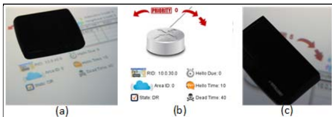
Fig. 5. a) Router specific information which is digitally embodied within the tangible device. b) Representative images are further used to simply the association and understanding of device parameters. c) Priority parameter on device is altered with physical rotation
