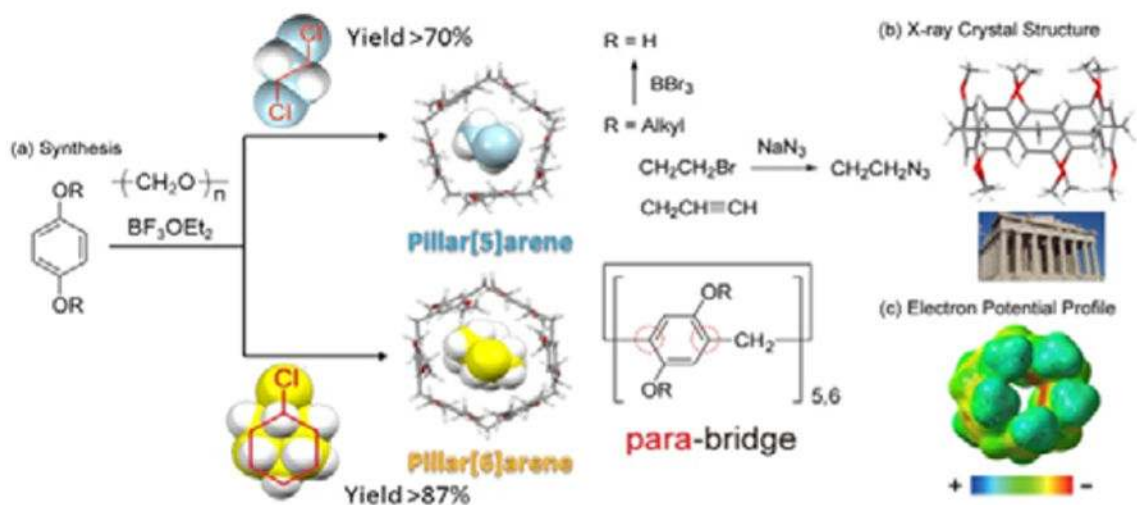
Fig. 9. (a) Synthesis of pillar[n]arenes with functional groups, (b) X-ray crystal structures of pillar[5]arene and (c) calculated electron potential profile (DFT, B3LYP/6-31G(d,p)) of a pillar[5]arene bearing 10 methyl substituents.
