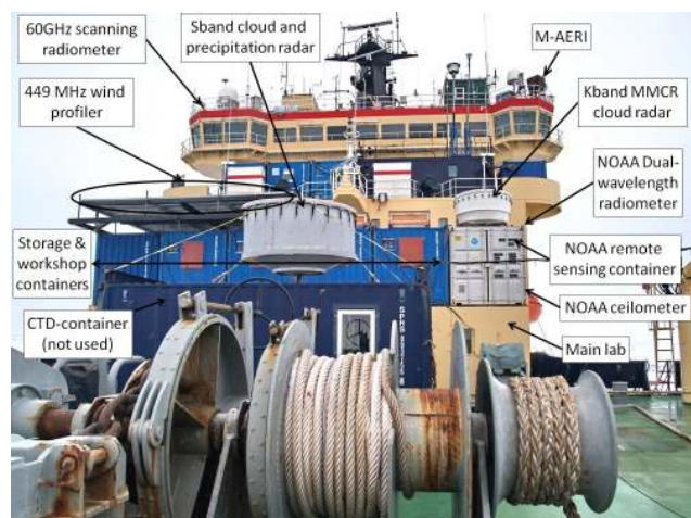
Fig. 5. Photograph from Oden 's foredeck showing the location of the surface-based remote-sensing systems. The dual-wavelength radiometer and the NOAA ceilometer are obscured behind the remote-sensing container.
