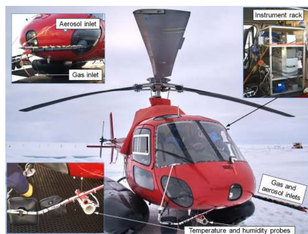
Fig. 10. Photograph of the helicopter that was used for vertical profiling, outlining some of the installations to sample meteorology, aerosol particles and trace gases.
