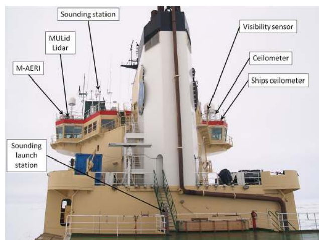
Fig. 7. Photograph of the installations on Oden as seen from the helicopter landing pad, which was also the sounding launch station; also seen are the location for several other instruments at the aft of the seventh deck.
