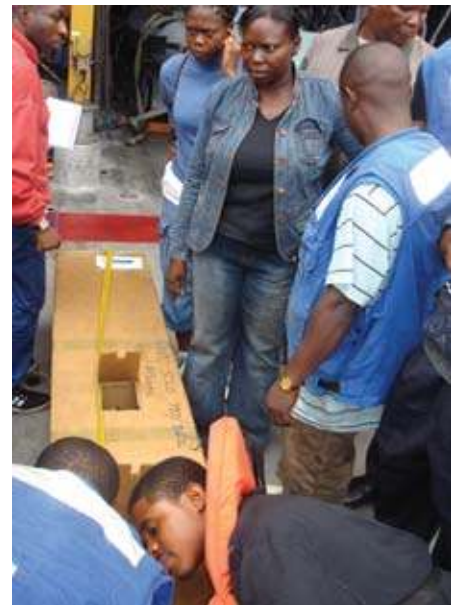
Figure 5. Participants of the training organized by the South Atlantic Argo Regional Center onboard the US Navy vessel HSV-2 Swift listen for pump sounds during predeployment testing of an Argo float. Photo by Augustus Vogel, US Navy
