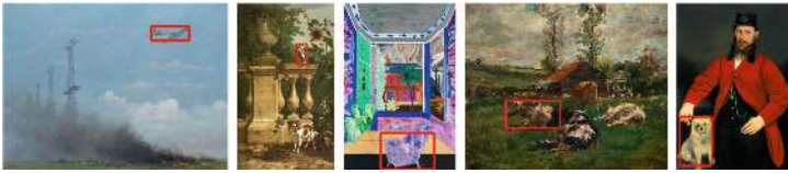
Fig. 5. Example detection windows obtained using the Faster R-CNN network. From left to right: aeroplane, bird, chair, cow. Only, the highest ranked window is shown in each image, even though multiple successful detection windows may have been found. Notice that very small objects are captured, such objects are often missed by an image-level classifier.
