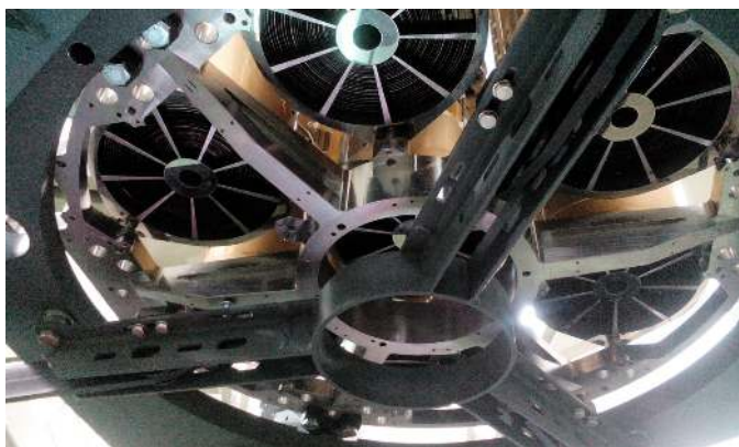
Fig. 4. Mirror systems installed at the assembly stand.
