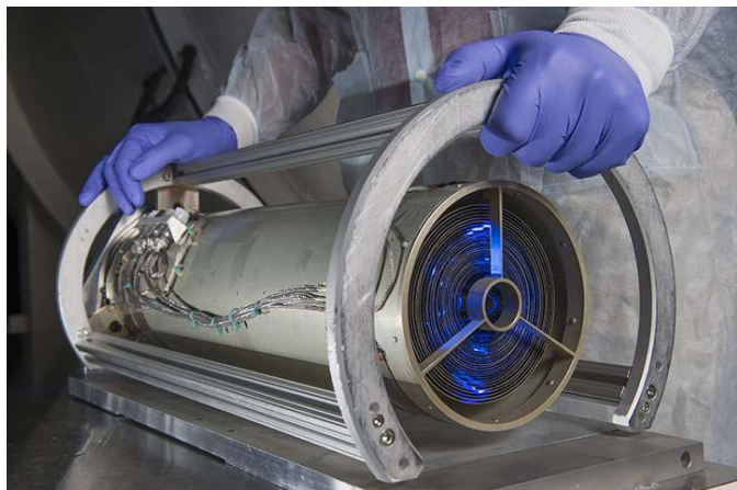
Fig. 2. One mirror system being prepared for testing at the MSFC Stray Light Test Facility.
