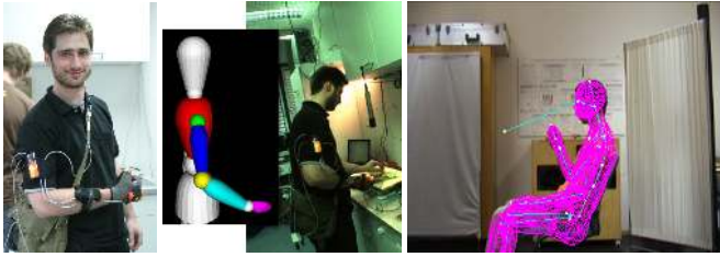
Fig.6: Sensing, reaching, and grasping activities using tiny inertial measurement units (left). Estimating the pose of people by accurately matching digital human models into image sequences (right).
