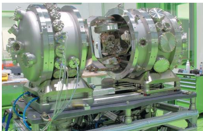
Figure 2 Reflectometer vacuum chamber opened to show the UHV-optical bench. The light comes from the left side.
