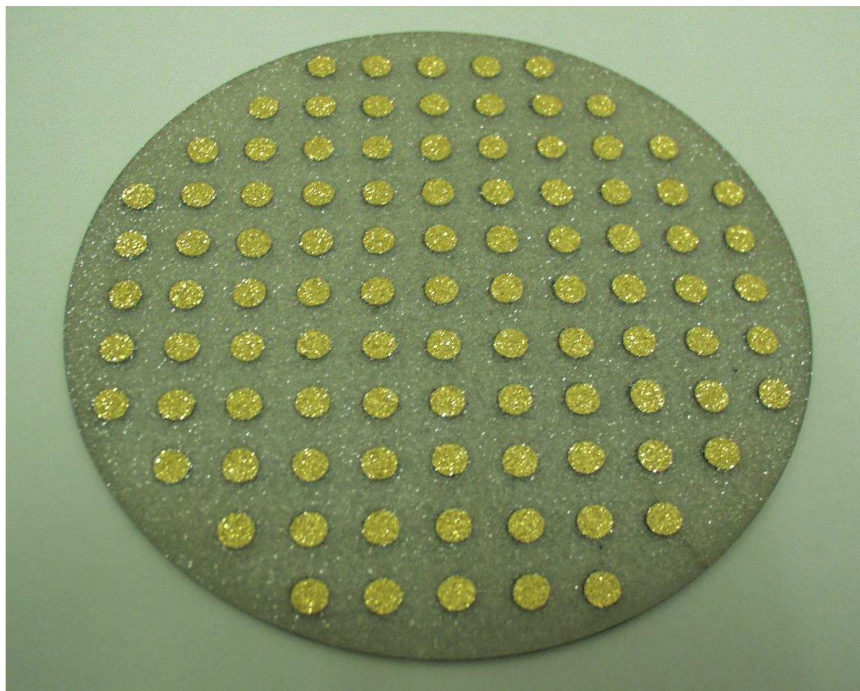
Figure 3. A 13cm diameter wafer of polycrystalline CVD diamond prior to dicing the BCM sensors.
