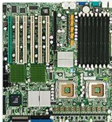
SuperMicro X7DB8-X MB with 2 * 2.66 GHz quad core Xeon and RAM @ 667 MHz
