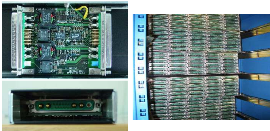
Figure 24. PP3 pictures. Top view with metal box open (top), the yellow wire connects the metal box to the cable shield. Front view of the PP3 (bottom), the two C-section pieces protect against magnetic fields. PP3 rack before cable installation (right).
