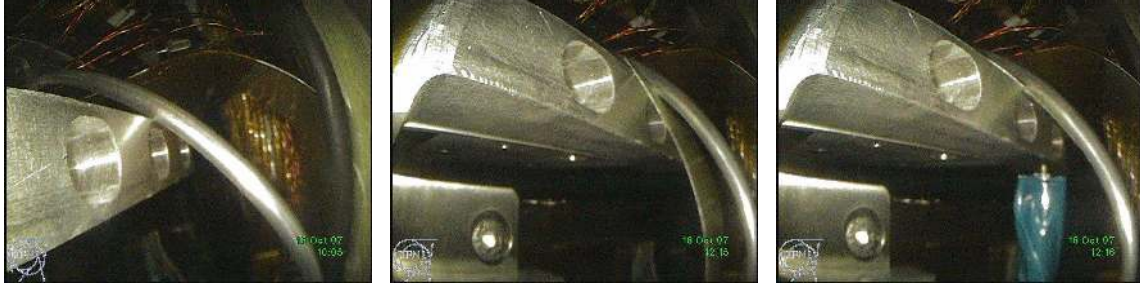
Figure 29. Short before any intervention (left). G10 being inserted between the endcap foot and the barrel pipe (centre). G10 inserted (right) and separated from the extender arm (with blue tape).
