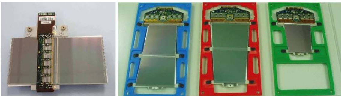
Figure 2. Picture of a barrel module (left). Three different types of endcap modules (right).
