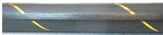
Figure 3. The TRT straw made from multilayer Kapton films and reinforced with carbon fibre bundles.
