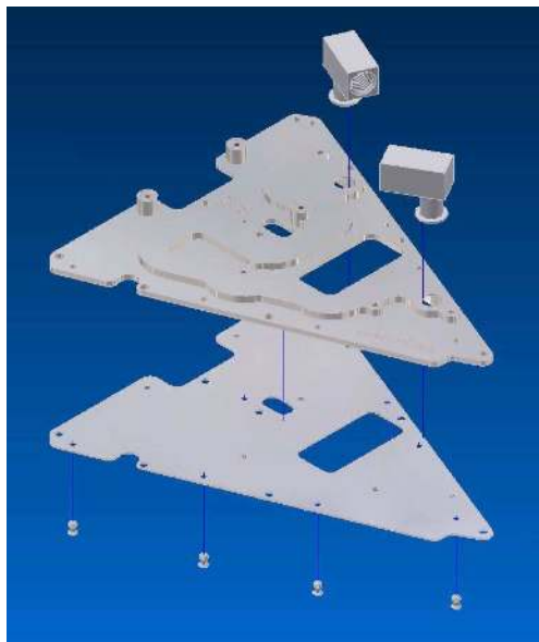
Figure 18. Exploded View of Cooling plate.
