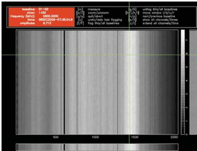
Figure 18. Screen-shot of the new PGFLAG task in the MIRIAD software package (see Section 5.2).
