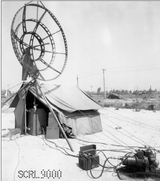
Figure 4: An AN/TPS-3 radar in operation in 1944 (courtesy CE LCMS Historical Office Department of the Army, USA).
