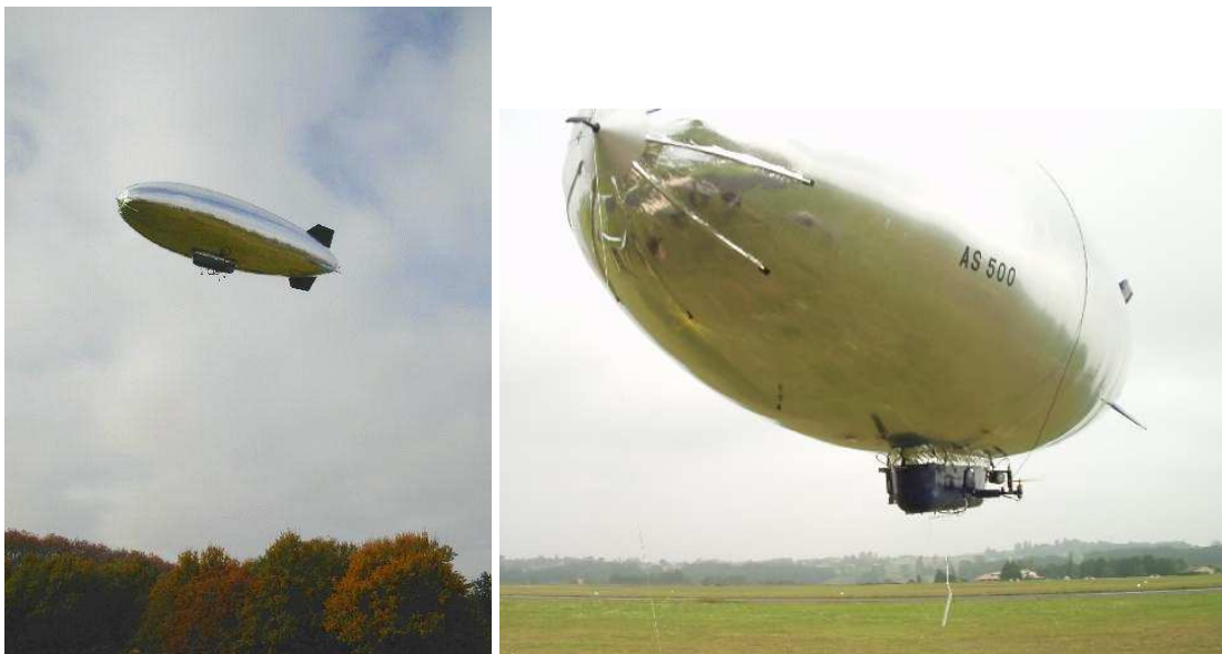
Figure 1: Karma during its maiden flight in November 2001 (left, no on-board instrument were installed at that time), and during test flights in summer 2002 (right - the cameras and the Ethernet antenna are visible).
