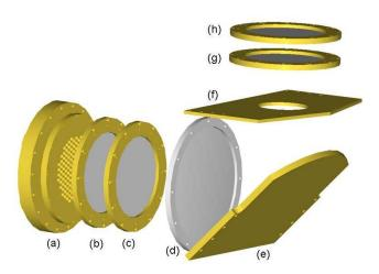
Figure 3. An exploded layout of the internal AzTEC optics. Components are: (a) integrated detector array, backshorts, and conical feedhorns (250 mK); (b) 310 GHz low-pass filter (250 mK); (c) 360 GHz low-pass filter (250 mK); (d) bi-convex ultra-high molecular weight polyethylene lens (4 K); (e) folding flat (4 K); (f) 50 mm diameter Lyot stop (4 K); (g-h) 390 GHz and 1050 GHz low-pass filters (4 K). Not shown are an additional 77 K 540 GHz low-pass filter and a Zotefoam PPA-30 cryostat window.
