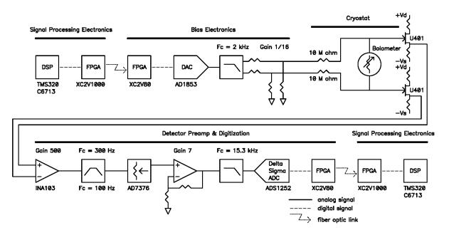
Figure 5. Schematic of the detector readout chain. All analog electronics are replicated 144 times in the sysem.
