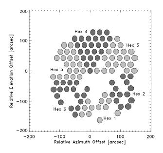
Figure 11. AzTEC's "footprint" on the sky at the JCMT05B run. The six hextants are labeled "Hex" 1-6. The alternate shading indicates which bolometers are located in each hextant. The size of the ellipse corresponds to the bolometer's FWHM, measured in the azimuth and elevation directions.
