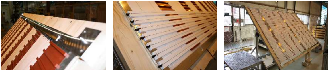
Figure 2: Scintillator modules assembly. Left) top of front half-module showing vertical bars, and the spacers-ladders that hold horizontal bars in place. Middle) rear half-module showing horizontal bars on their ladders. Right) Assembled rear half-module, the front half-module can be seen in the background.
