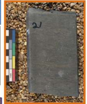
A – Brachiopod-rich silty dolostone. Bioturbated in some areas. Contains crinoids and echinoderms fragments Average Porosity: 4.5%
