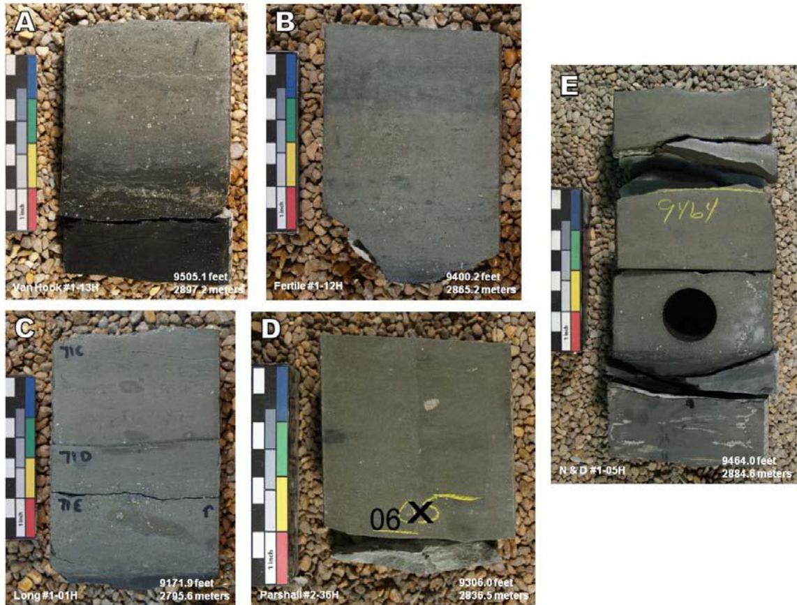
Figure 2. Core photos of facies A – muddy lime wackestone. Crinoid and brachiopod shell fragments are more concentrated at the base of the facies. This lowermost facies of the middle Bakken lies directly above the contact with the lower Bakken shale as seen in photo A.
