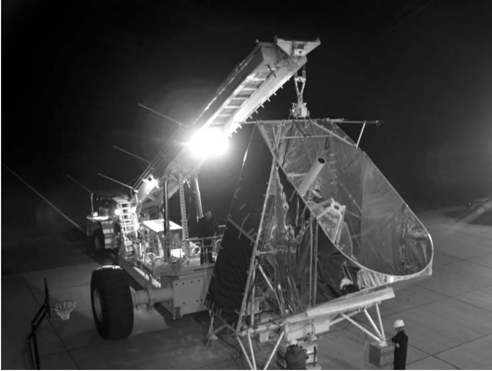
Figure 11. The BLAST gondola prior to launch from Ft. Sumner, NM in September of 2003. The cable suspended gondola design is lightweight, has a high tensile strength, and a high resonant frequency.
