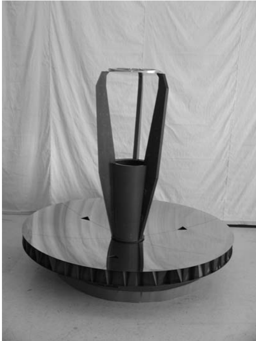
Figure 5. The BLAST mirror. The 2 m diameter carbon fiber mirror is made by Composite Optics Incorporated. It weighs 32 kg and has a surface rms of 2.4\mu\text{m} .
