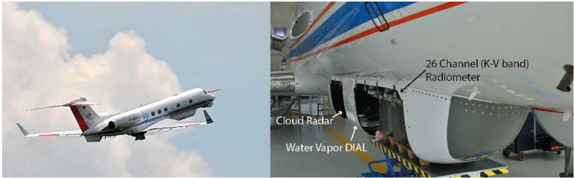
698 FIG. B1. HALO with the remote sensing bellypod mounted to its fuselage, left. Closeup image of belly pod 699 showing three compartments for Cloud Radar, water vapor lidar and three bank, 26 channel radiometer.
