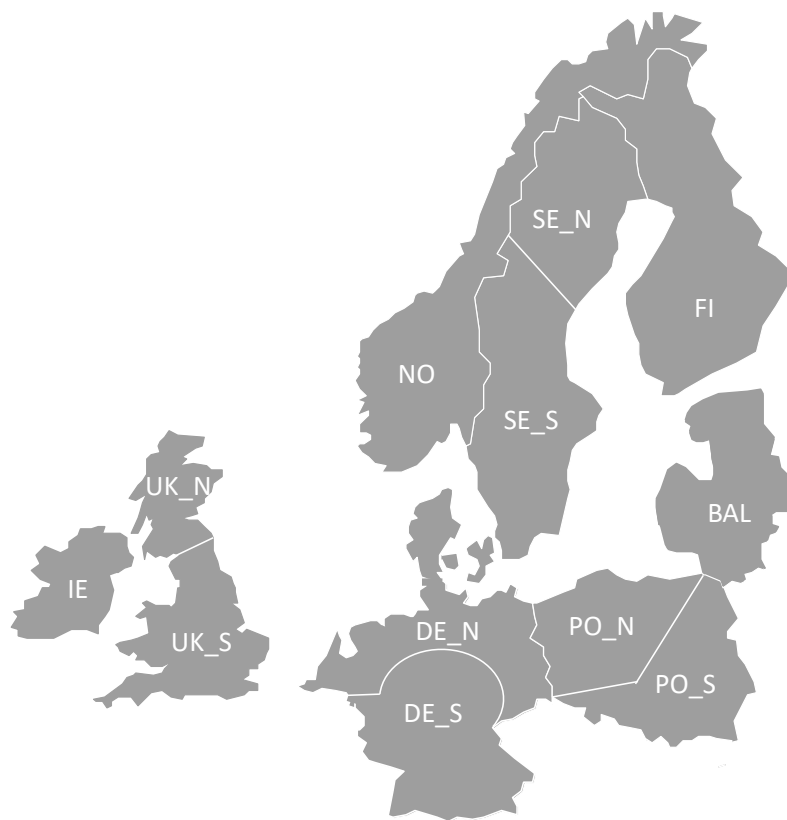
Figure A1. Map of regions considered in this work. Northern Europe is subdivided into 12 regions based on major bottlenecks in the transmission grid and key differences in renewable resources.
