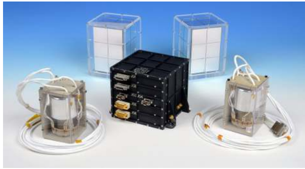
Fig. 1 Sensor flight models (left and right in front) with electronics box (black, center) and the thermal housing (in the back)
