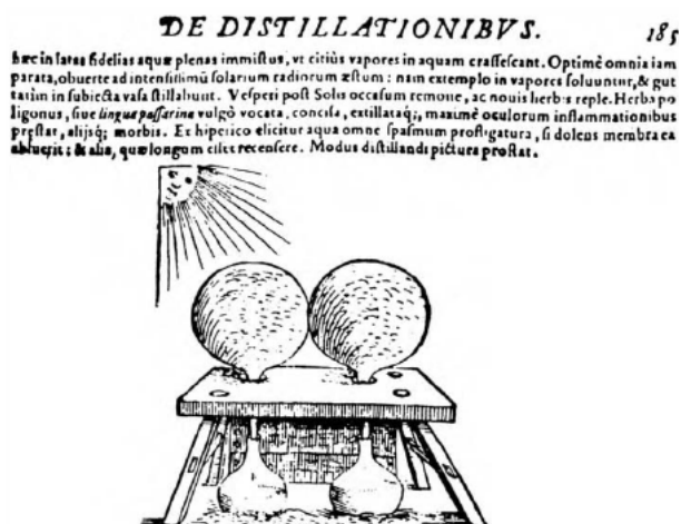
Figure 11. The first historically known solar distillation equipment, according to Giovanni Batista De La Porta; the sun evaporates the water inside the glass vessels and distilled water is collected beneath the vessels [86].
