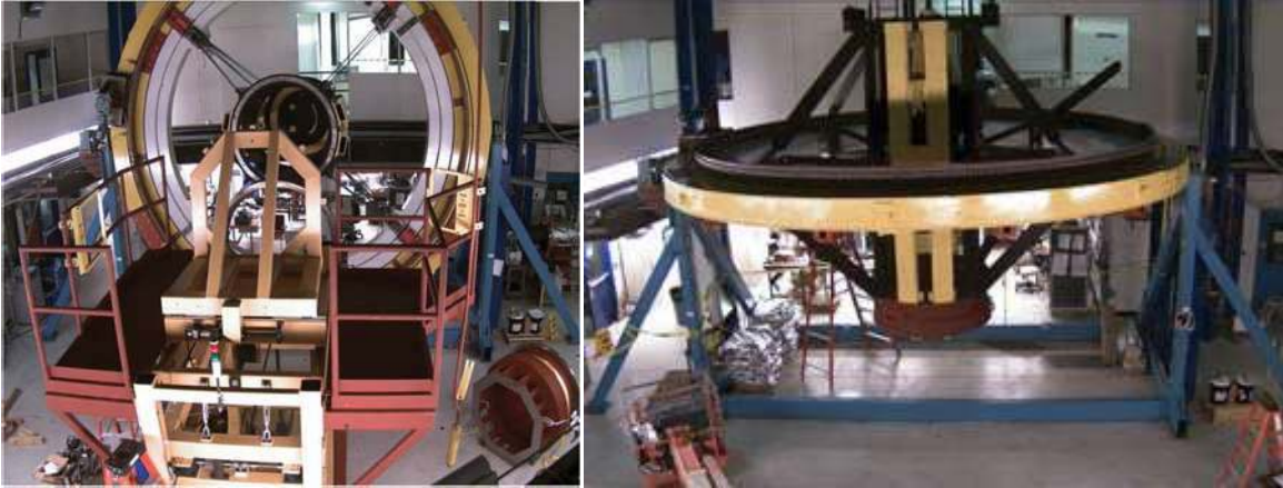
Figure 5.10: The telescope simulator at Fermilab with the DECcam Prime Focus Cage. The structure in the background supports a copy of the two rings (white) at the top of the Serrurier Truss. The yellow rings are connected to motor drives that enable the Prime Focus Cage to be pitched and rolled, for the purpose of testing and pre-commissioning of the instrument prior to delivery to the telescope. The foreground structure (left) is the secondary (f/8) mirror handling fixture, enabling the installation of the mirror over the end of the optical corrector for the use of instruments at the Cassegrain Focus.
