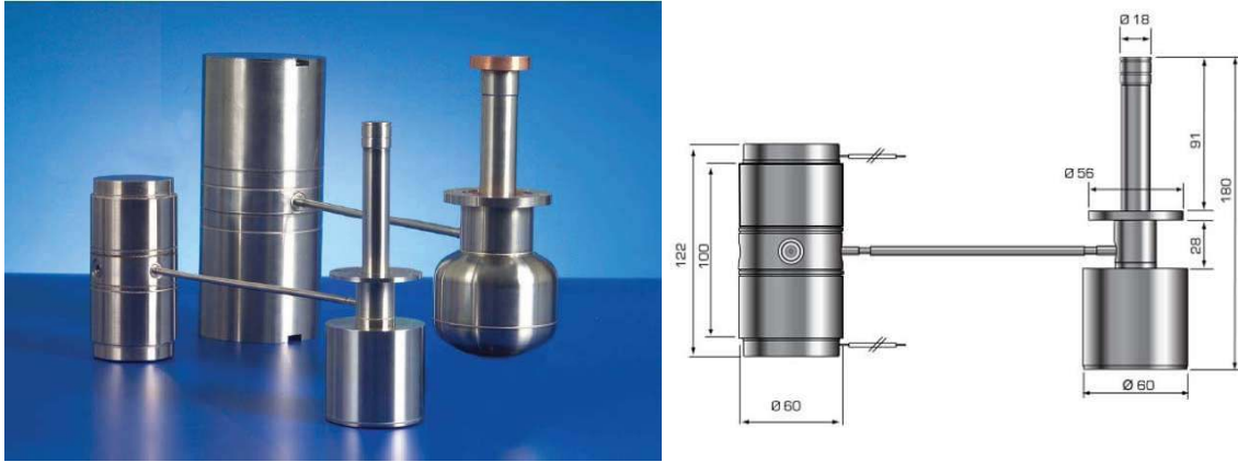
Figure 5.43: Left: two models of LPT, LPT9510 (in the foreground) and LPT9310, with powers of 1 W and 4 W at 80K, respectively. Right: dimensions of the LPT9510 model.
