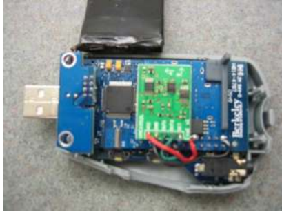
(a) A two-axis magnetometer is attached to a Tmote Invent via its ADC.
