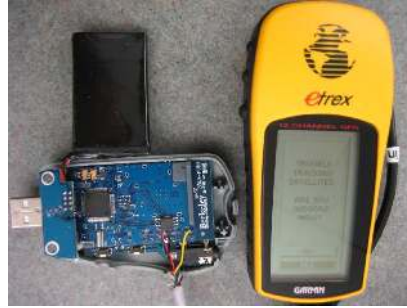
(b) An external GPS unit is attached to a Tmote Invent via its UART0 port.
