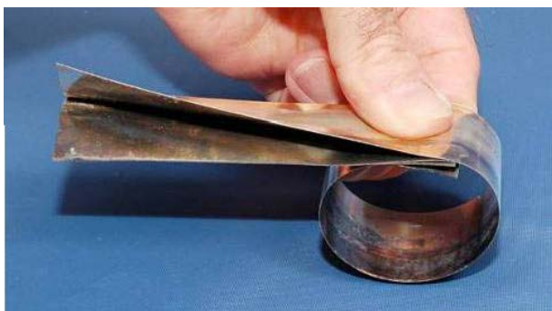
Figure 2-2: Folding of a TRAC boom sample [7].
