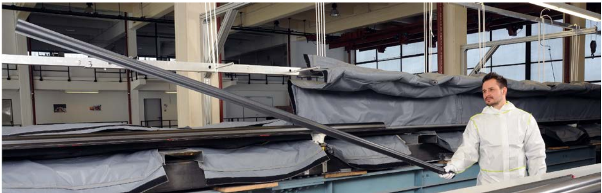
Figure 6-1: DE-ORBIT SAIL boom of 3.6m length self-supporting under gravity.
