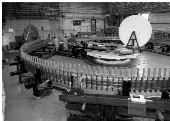
Fig. 7. The coil winding fixture, shown on the turntable. An inner coil is being wound.
