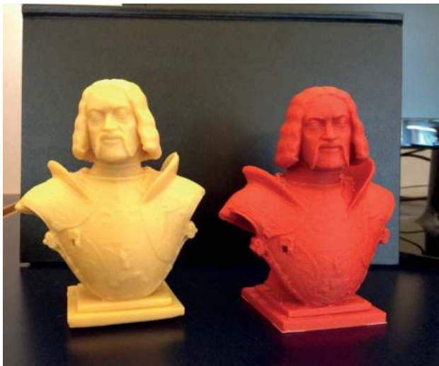
Figure 8: Resin (yellow) and ABS (red) 3D sculpture printed at scale 1:5
