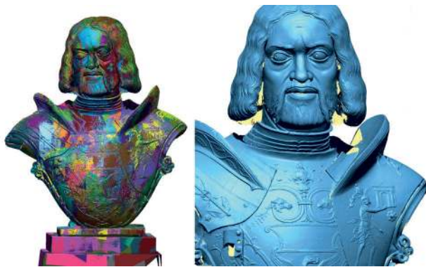
Figure 4: the model 2 made by each single scan and then merged in a single mesh. The missing part in yellow are evident and they are concentrated in the area under the head of hair.
