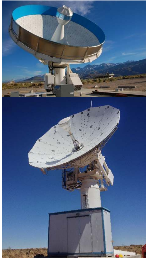
Figure 3. Top: The C-BASS North telescope, located at the Owens Valley Radio Observatory in California, U.S.A. Bottom: The C-BASS South telescope, located in the Karoo desert, South Africa. The weather shield around the receiver is removed in this image, showing the lower part of the feed horn and cryostat.
