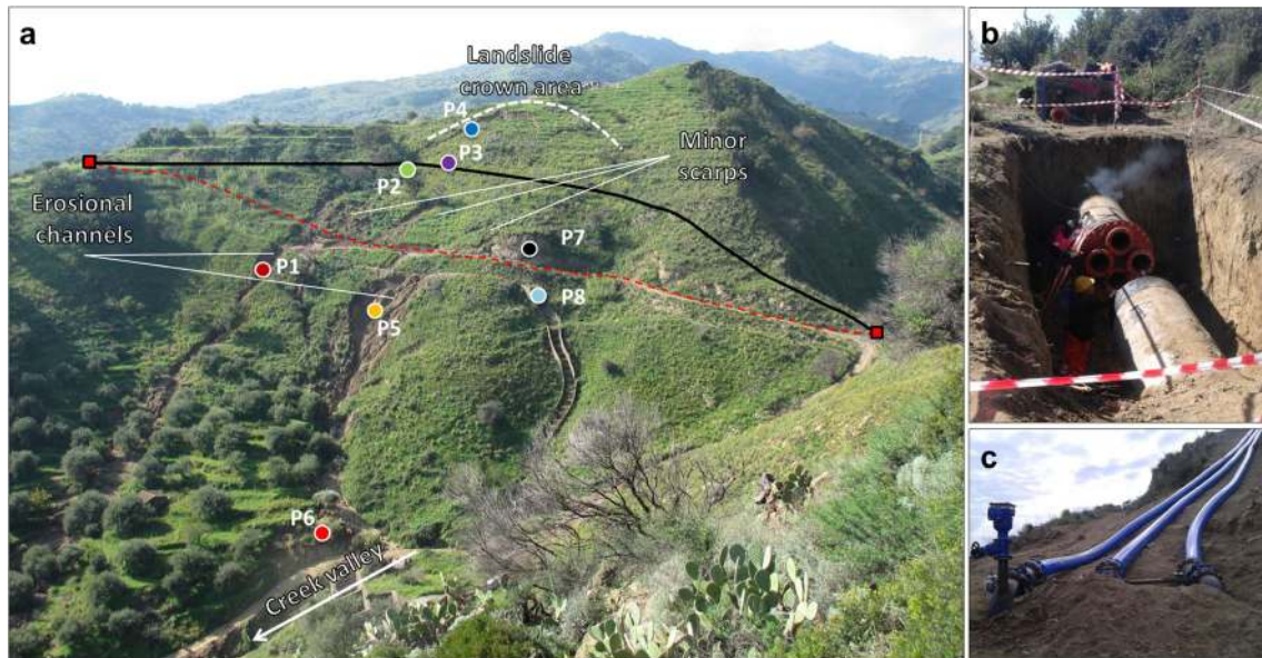
Fig. 3 a Image of the Calatabiano landslide acquired on 10 November 2015, from the monitoring system installation point. The dashed white line represents the main landslide crown, the dashed red line represents the interrupted pipeline (b), and the black line represents the new pipeline by-pass (c). P1–P8 represent the GB-InSAR monitoring points
