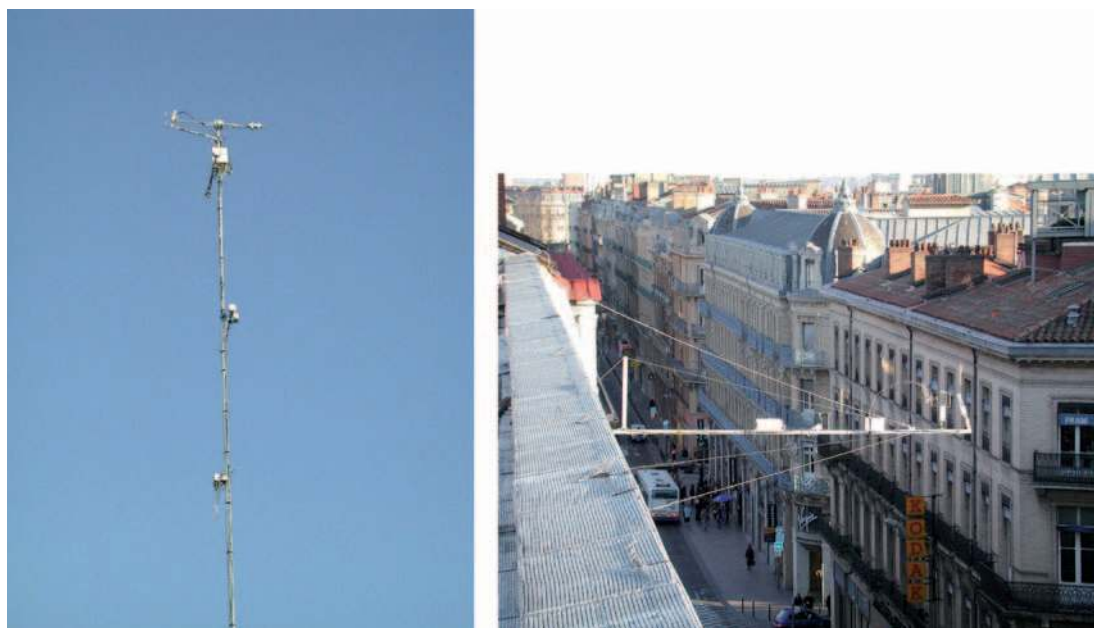
Fig. 4. Left: the pneumatic tower for surface energy balance observations; Right: 5 m turbulence-aerosol measurement boom at the top of Alsace-Lorraine street canyon
