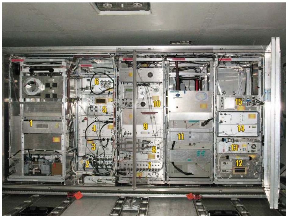
Figure 1. Frontal view of the container inside the forward cargo bay of the A340-600, facing the flight direction. Its width is 3 meters and its mass is 1.5 ton. In-flight its doors are obviously closed. 1. PTRMS. 2. Main power unit. 3. Aerosol, CPC and sampler. 4. Aerosol, 2 CPCs. 5. Aerosol OPC. 6. DOAS. 7. Base power unit. 8. Water total and vapor. 9. Mercury. 10. Ozone fast and standard. 11. NO and NO y . 12. CO 2 . 13. CO. 14. O 2 . 15. Master computer. At the rear, the 2 air sampling units, air pumps, a VOC sampling unit, calibration and working gas supplies are accommodated.
