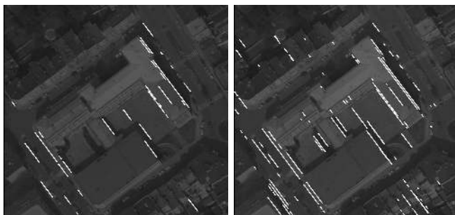
Figure 6: a/ Line segments belonging to the same direction as the walkway (left) b/ idem, after adapting the orientation of the lines such that they pass through the vanishing point (right).
