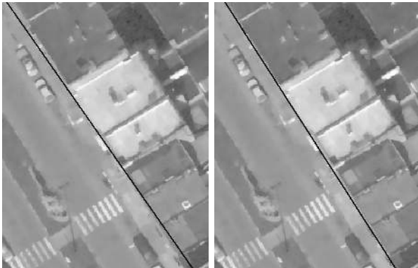
Figure 9: The original Hough line (left) and the line through the vanishing point (right).
