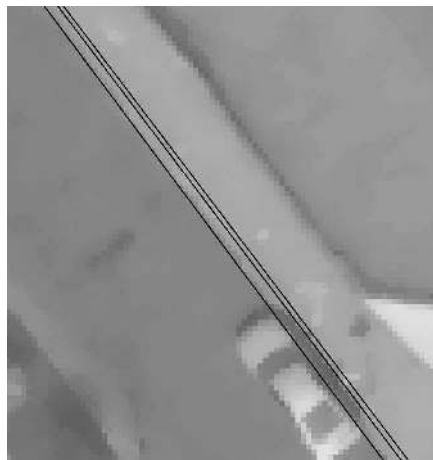
Figure 7: A detail of fig. 3 with the three lines fitted to the walkway: from top to bottom the Hough line, the line with average orientation and the line through the vanishing point.
