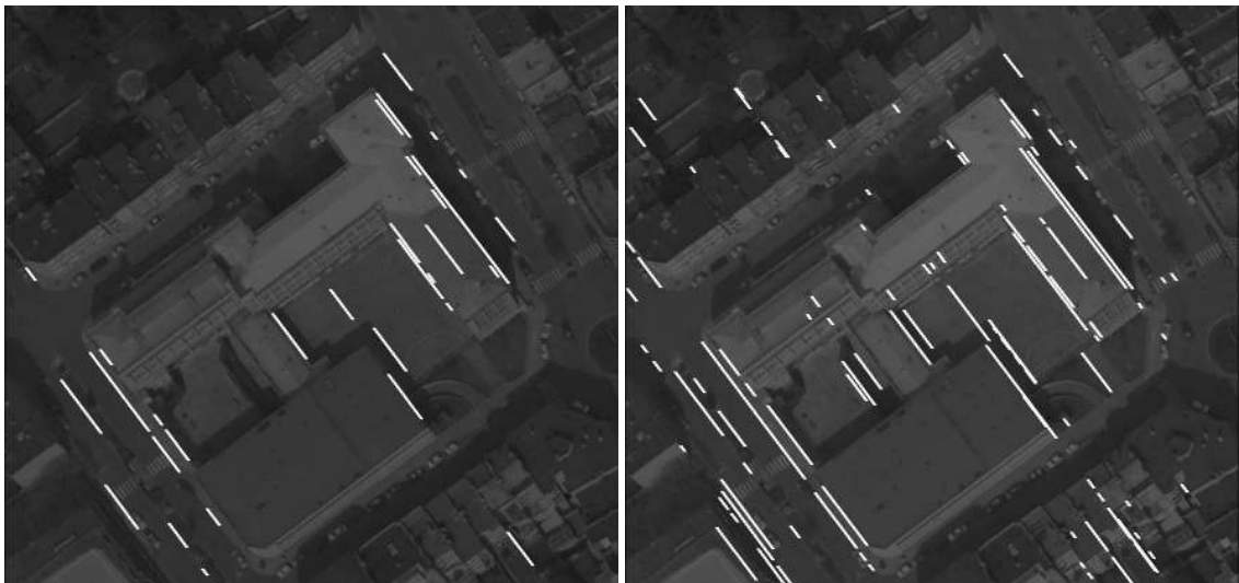
Fig. 9. a/ Line segments belonging to the same direction as the walkway (top) b/ idem, after adapting the orientation of the lines such that they pass through the vanishing point (bottom).
