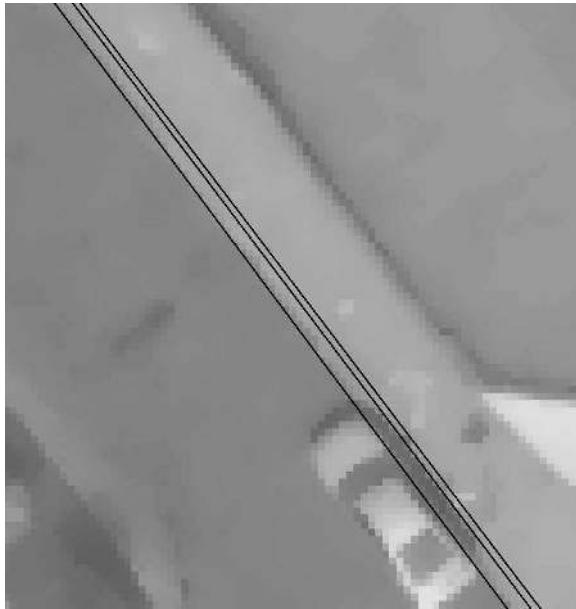
Fig. 8. A detail of Fig. 5 with the three lines fitted to the walkway: the Hough line at the right, the average line in the middle and the line through the vanishing point at the left.
