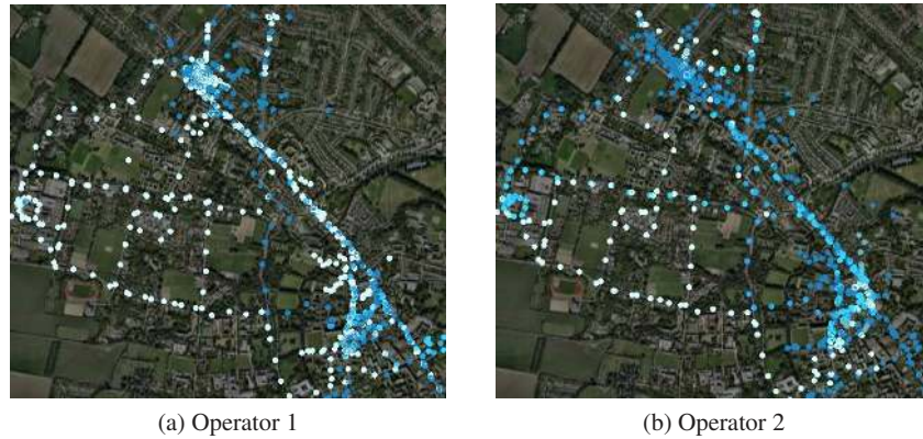
Fig. 4: Signal strength perceived by two identical co-located handsets in several locations in west and centre of Cambridge (UK) with different network operators. Lighter points indicate better signal strength.
