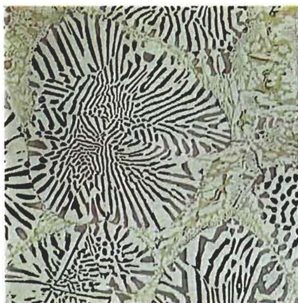
The eutectic structure of a low temperature silver brazing alloy containing 12.5 per cent gold. This has a liquidus of 660°C and a solidus of 630°C × 125
