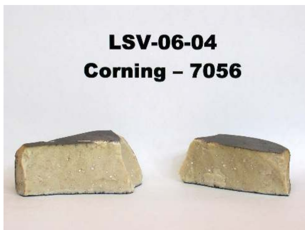
Figure 12. Photograph of CWF showing a fairly homogenous matrix with only minor inclusions, which may be unconverted zeolite.
