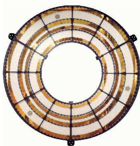
Fig. 12.— Photograph of the HETG. Glittering gold, the 336 grating facets are visible mounted to the black-anodized support structure, the HES. The outer two rings of gratings are MEGs and intercept rays from the HRMA shells “1” (outer most) and “3”; the inner two rings are HEGs and work with HRMA shells “4” and “6” (inner most.)
