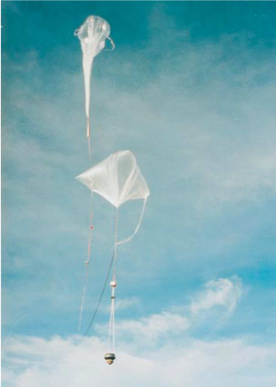
Figure 14. Ascending phase of the COMAS SOLA balloon flight. The secondary balloon, which is lifting the probe mock-up, will be released later on, and the payload will continue its ascent dragged by the primary balloon. A damper has been fixed under the mock-up in order to damp the landing.
