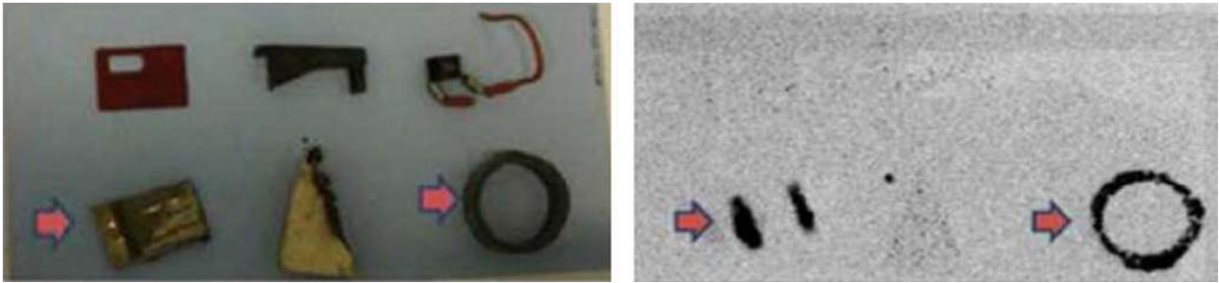
Fig. 9. Measurement of tritiated waste by digital autoradiography.
