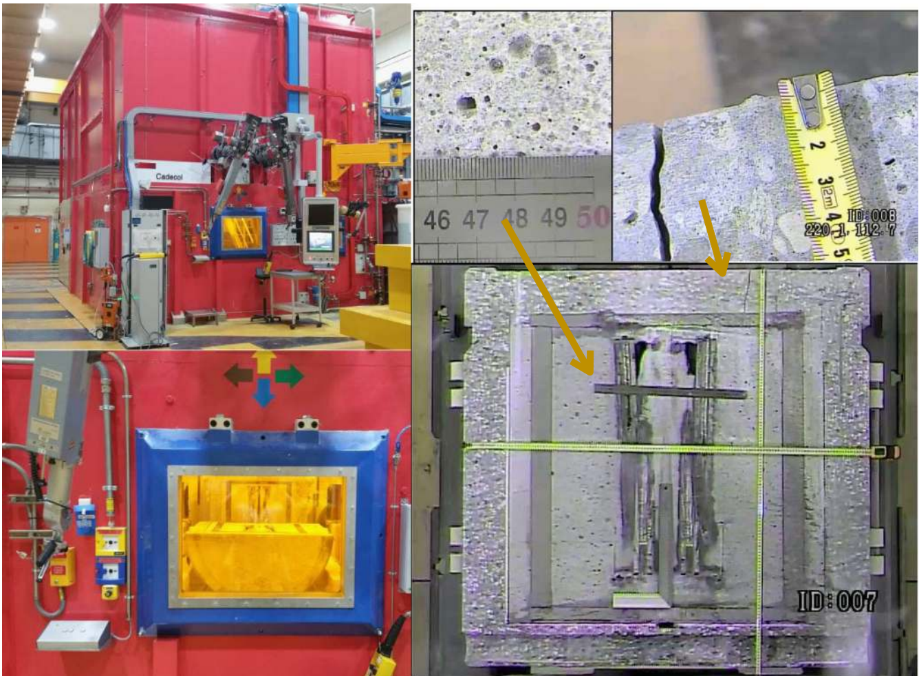
Fig. 23. Expertise of a heterogeneous hull (cutting of a 5 m 3 concrete package by wet process) in the CADECOL cutting and coring hot cell, in CHICADE basic nuclear facility, at CEA Cadarache.
