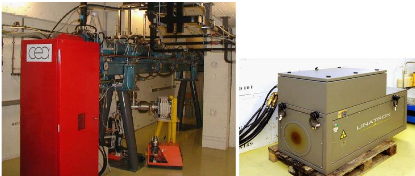
Fig. 18. The SAPHIR facility of CEA LIST makes it possible to characterise waste packages by photofission (A. Gonin/CEA). Left: 15 MeV LINAC. Right: 6/9 MeV LINAC.
