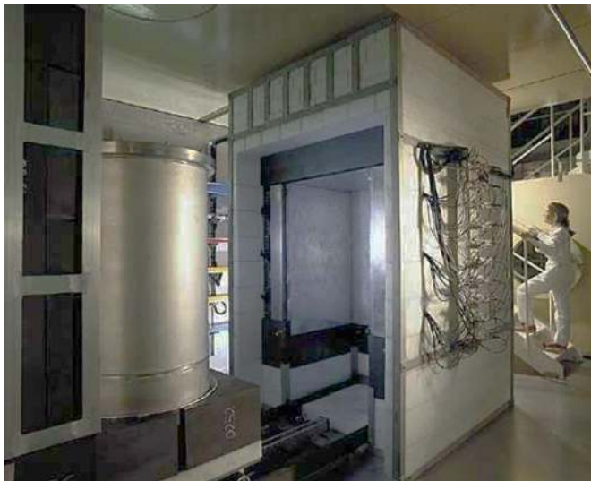
Fig. 29. CHICADE's graphite neutron measurement cell for 200 L drums SYMETRIC, including 99 ^3\text{He} proportional counters with charge preamplifiers connected to an electronics counting coincidences between spontaneous fission neutrons (passive mode) or prompt and delayed fission neutrons induced by the use of a 2 \cdot 10^9 \text{ n.s}^{-1} high flux neutron generator (active neutron interrogation).
