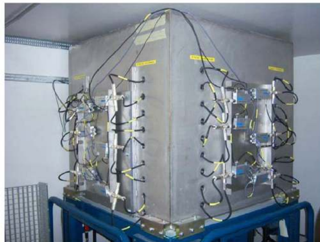
Fig. 8. Photograph of the neutron measurement station at the PEGASE facility in CEA Cadarache and simulation model with a Monte Carlo neutron-gamma transport code, showing a calibration drum filled with inactive materials representative of the waste matrix and hollow tubes to introduce radioactive sources ( ^{252}\text{Cf} , AmBe) or Pu samples (calibration standards).
