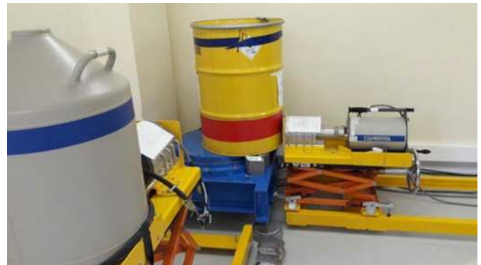
Fig. 3. Gamma spectroscopy station for 100 to 200 L waste drums, in CHICADE basic nuclear facility, at CEA Cadarache.
