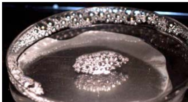
Fig. 1. Bubbles floating on water in a petri dish. The bubbles are observed to aggregate before moving to the wall of the container. After sufficiently long times, the island of bubbles in the center also migrates to the wall.
