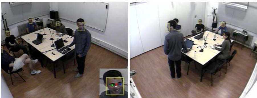
Fig. 5 Example of video annotations for an interactive seminar in the UPC smart room. Face bounding boxes and facial feature annotations are depicted for two camera views
