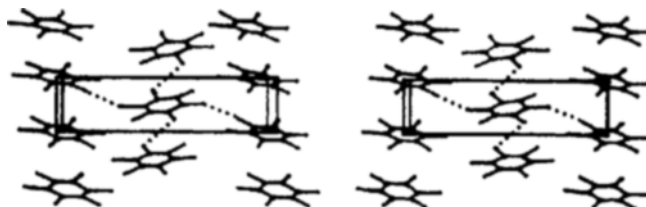
Figure 3. Stereoview of the crystal structure of hexachlorobenzene (HCLBNZ). Notice the linear ribbons interconnected by Cl . . . Cl contacts.
